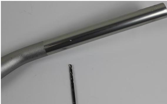
Once the correct position of the manual instruments has been found, they must be screwed. Mark (slightly drill) the hole. To make sure that the hole is centered on the handlebar (diameter 4mm), we recommend dismantling the handlebar again and drilling the hole for the clutch and brake fittings on a pillar drill.
